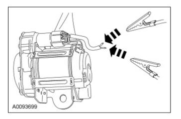
8. NOTE: Make sure to maintain the connections to the safety belt buckle or retractor.
